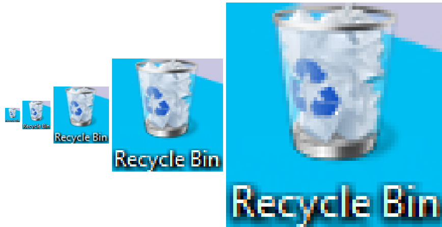
Figure 3.6: Example of how template size variance affects a image for the values 0.25, 0.50, 1.0, 2.0, 4.0 respectively
