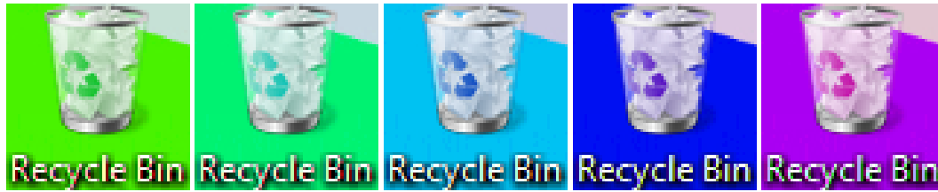
Figure 3.3: Example of how colour variance affects a image for the values -90, -45, 0, 45, 90 degrees respectively
